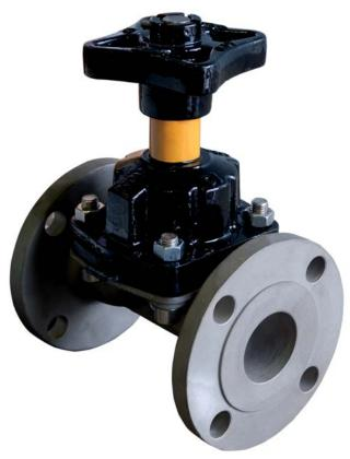
KDV's range of bi directional Weir Type diaphragm valves offer exceptional durability and reliability. The clean design completely isolates line media from the mechanical components of the valve. Bubble tight shutoff (Class VI) and in-line serviceability (top entry) maximise plant efficiency and productivity.
