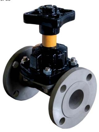
KDV's range of bi directional Weir Type diaphragm valves offer exceptional durability and reliability. The clean design completely isolates line media from the mechanical components of the valve. Bubble tight shutoff (Class VI) and in-line serviceability (top entry) maximise plant efficiency and productivity.
